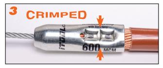
Use the WCT 1000 tool, or similar 12 ton die crimping tool, to squeeze the crimp head in one or two positions depending on the iTOOLco specifications.
